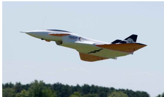
Fig. 4 Our 24.9 kg UAV ISAAC during a test flight.
