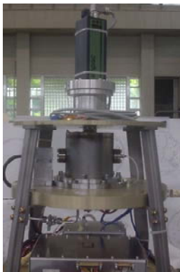
Fig. 1 Experimental apparatus of diamond synthesis installed on the sounding rocket top
