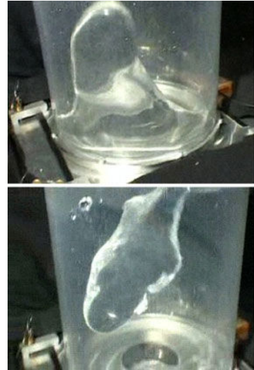
Fig.2: Water floating in a water repellent coated plexiglas cylinder.
