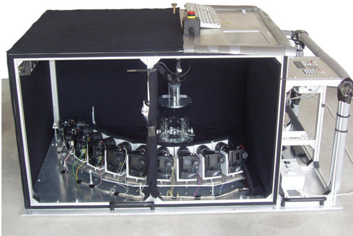
Fig.1: "Frozen Reality" experiment setup. Ten cameras are directed to an exchangeable experiment cylinder. A projectile will be automatically accelerated with a spring
