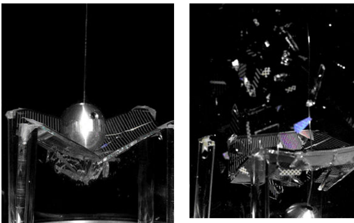
Fig.4: Impact of a metal projectile in a solar panel with force of gravity (left), and in weightlessness (right)
