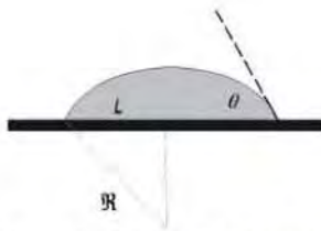
Fig. 1. Partial wetting case. The contact angle \theta is measured inside the liquid, R is radius of the drop and L is radius of the drop base on the solid substrate.
