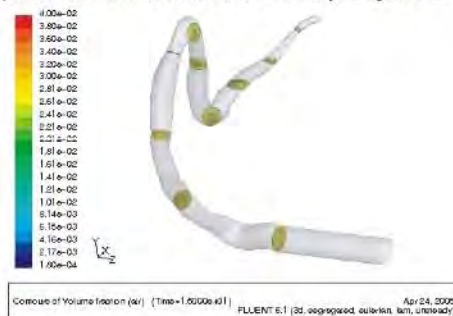
Fig. 3. Contours of air volume fraction for pulsatile flow 0.6Lit/min, artery length 500 mm and diameter 5-20 mm, pulsation 60 bpm, 50% pulse amplitude, 3% air volume fraction. The picture refers to 300 μm bubbles
