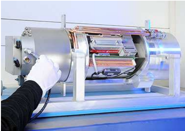
Figure 2: Compact and fully MSL compatible 110 kV X-ray radiography insert for in-situ monitoring of interdiffusion and solidification processes.
