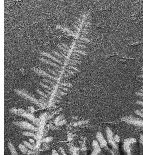
Figure 3: X-ray image of dendrite growth in Al-Cu sample during ground tests with XRMON-GF experiment to be flown on MASER 12 in November 2011.
