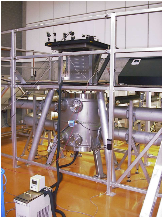
Figure 1: A picture of a 33 T poly-Bitter magnet. The magnet consists of 4 electrical coils, mounted inside a 1 m diameter, 1 m high cylindrical housing. At maximum field the electrical current is about 37000 A using a power of 17 MW. The magnet is cooled by cold water (12 °C) at a flow of 145 l/s. Access for samples and in-situ measurement equipment is possible from above and below the magnet, inside a 32 or 50 mm diameter vertical bore.
