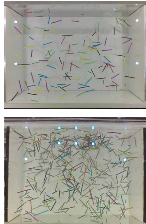
Figure 1: Top: Rod-like particle ensemble in very dilute limit (Knudsen regime), image from the drop tower microgravity experiment. Bottom: rod-like particle ensemble with higher volume fraction beyond Knudsen regime, image from Blue Origin suborbital flight microgravity experiment.
