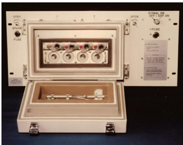
Incubator installed in Spacelab rack; beside the culture block syringes containing either activator, marker and fixative are placed.
