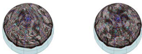
Figure 1. Sheet-like thermal flow in the GeoFlow I spherical experiment with silicone oil of temperature-stable properties (left, RaE=1.17 \cdot 10^6 ) and GeoFlow II experiment using a fluid with temperature dependent viscosity and volume expansion (right, RaE=1.87 \cdot 10^6 ).
