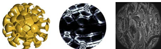
Figure 2. Sample of numerical model for plume-like upwelling thermal flow with no-slip conditions, 1/r_5 buoyancy for Ra_{centr}=6.42 \cdot 10^4 , viscosity contrast \mu=103 .
